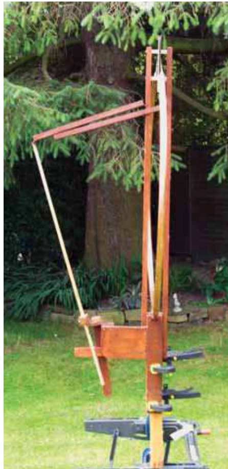
PHOTO 3: The mechanical tuning arrangement set so that capacitor plates are close together for the 30 and 40m bands.
