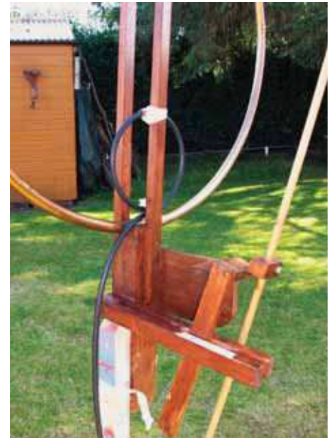
PHOTO 4: The Faraday coupling coil and the fine-tuning lever in more detail.
