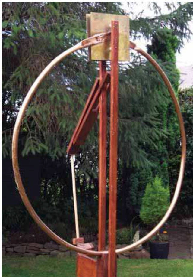
PHOTO 1: The overall construction of the 'Joiners Delight' antenna. The element is made from a 3m length of 22mm copper tube bent into an approximate circle of approximately 950mm O/D.
